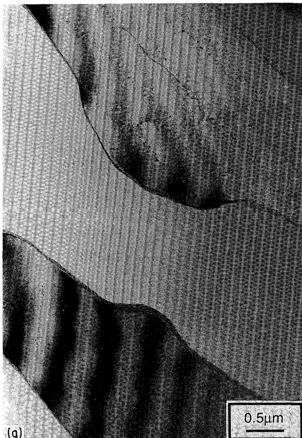
Figure 3 Structure within the thin region of PFC ribbon. Note the cellular morphology (a) and the presence of fine precipitation (b).
